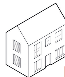
Inconsistent window treatment on different elevations
